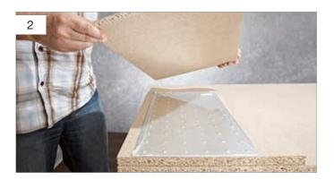
Delicate sheets are packaged in protective sheeting. Stick the sheet with the protective sheeting to the wooden board. This optimally protects it against scratches and makes it extremely easy to remove from the particle board once it has been worked.
