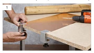
If you want to bend a metal sheet to form a rounded structure, round timber in different diameters is the perfect solution. For the sheet to be bent exactly parallel, it must not slip during the powerful bending process. To this end, you must ensure that it is firmly clamped on the edge of the workbench (e.g. with **alfer** multi-clamps or other vices).
