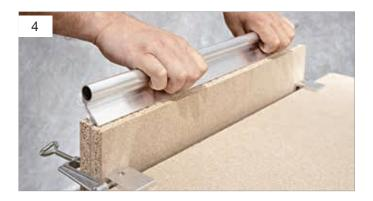
For the subsequent bend we recommend using a profile, roof strip or board to bend the projecting sheet forwards (towards the body) as uniformly as possible until it reaches the desired bend angle. If you do not want to bend just one angle, but rather create a U or Z-shaped sheet, simply repeat the process on the other side of the sheet.
