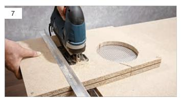
For straight cuts, you can screw on an aluminium bracket as an end stop for a super-straight cut.
