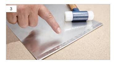
Next, anchor the sheet flat to the workbench and carefully tap down the short strip of sheet along its full length. The small sheet deformations do not impair the appearance of the finished product as they are on the underside of the sheet.
