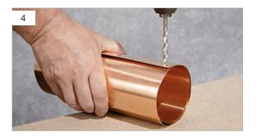
You can now push the sheet into itself until you have created the precisely desired diameter. Next, fix this diameter by riveting, soldering, bonding or welding the sheet.
