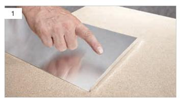
Crimping means that a narrow sheet edge is folded back on itself by a full 180°. This creates an elegant and effective edge guard and stabilises the sheet to prevent it from sagging.
