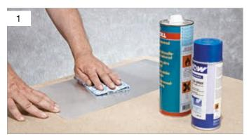
Metal sheets can be successfully painted. We recommend car spray paints because they ensure a uniform coat of paint and good bonding. Before painting, the sheets must be clean, free of grease and dust and totally dry.
