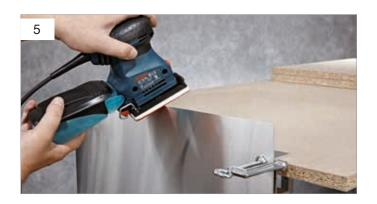
For the final smoothing stage, remove the sheet from the sandwich and clamp it without the particle boards. Next, attach finely-grained abrasive paper to the orbital sander and move it over the sheet edge again at a flat angle.
