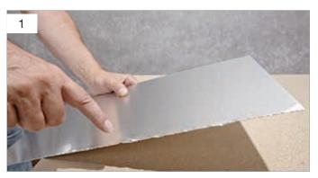
Professional tip: uneven, rough or even frayed sheet edges can be easily smoothed off lengthwise with an electric orbital sander. This applies to not only aluminium sheets but also steel ones.
