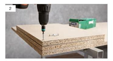
Screw or clamp the sheet between two particle boards in sandwich format (as in the cutting instructions above), ensuring that the uneven, rough edge of the sheet only protrudes 2–3 mm outside the particle boards. This reliably prevents the sheet from wobbling, bending or becoming scratched.
