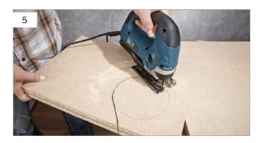
Now use the jigsaw to cut out your desired shape. We recommend working with a low stroke rate.
