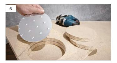
Here, you can see the perfectly round, non-scratched circular piece of the round studded sheet. Even on the studs, the jigsaw has not slipped from the cut line thanks to the guidance from the particle boards.
