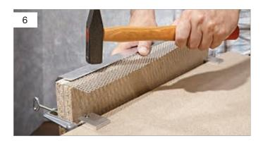
If you are unable to create the bend manually due to the sheet being too long (over approx. 80 cm) or too thick, you can also use a hammer and impact shield (profile or wood batten) to assist you and carefully tap the sheet down.
