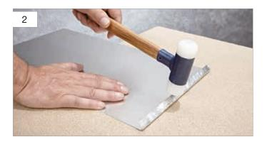
The procedure is the same as that described under 'Straight bends' on page 14 except that you only need a sheet to protrude by 10–15 mm in order to crimp the edge.
