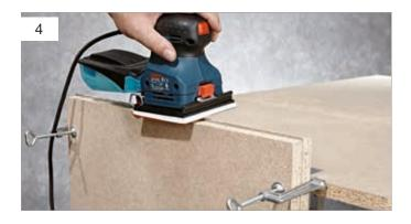
When sanding a very rough sheet edge, we recommend first using very coarse-grained abrasive paper with a high material removing effect. Sand the sheet until it has the smooth edge that you desire.
