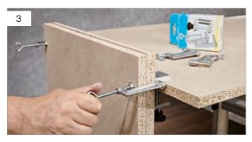
Clamp the 'sandwich' vertically in front of the workbench (ideally using an **alfer** multi-clamp) and guide the orbital sander evenly along the protruding sheet at high speed.
