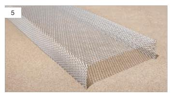
This image shows you the finished U-sheet. It is precisely flush, parallel and rectangular.
