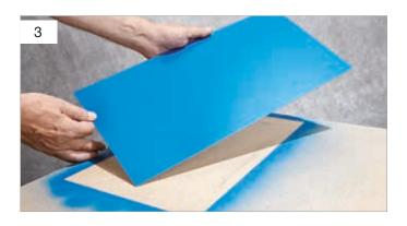
Tip: for the best results, apply the paint in multiple stages, leaving it to dry for at least 5 minutes between each application. This prevents paint runs and provides optimal paint coverage.
