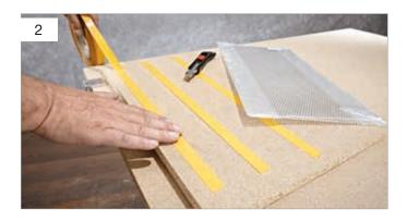
Tape the sheet with the protective cover onto a particle board with the bending edge lying precisely along the edge of the board. Next, place the second particle board flush with the bending edge and screw the two boards together outside the sheet.
