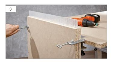
Use the **alfer**° multi-clamp to tightly clamp the sandwiched structure in front of the workbench.
