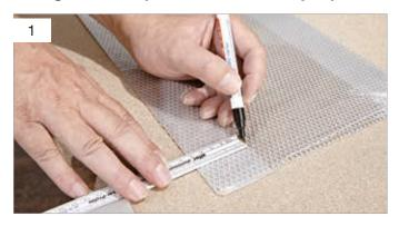
For straight bends, start by drawing your bending edge. We recommend leaving the protective cover on the sheet. This provides it with optimal protection and helps prevent it from being scratched while you work.
