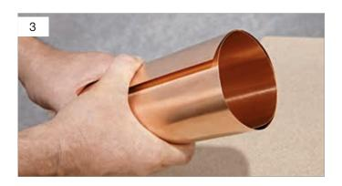
check this straight course by ensuring that the rolled sheet edge is always precisely aligned with the edge of the sheet still lying flat. Due to the spring recoil of the sheet you must rotate it about 1.5 times. On unrolling the round timber, the diameter of the bent sheet will expand by approx. 30%.
