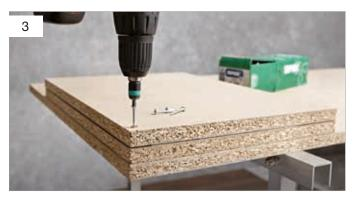
Now use countersunk screws to connect the two wooden boards. You can also drill through the part of the sheet that is not required and fix it with screws so that it cannot slip out of place.
