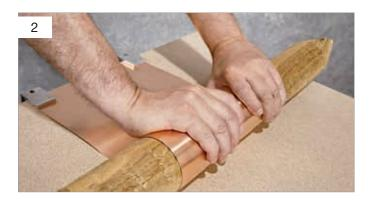
Always ensure that an exact right angle is formed with the longitudinal axis of the round timber! Next, roll the round timber towards yourself evenly and with a relatively high amount of force while also pushing it away from yourself, keeping it under pressure. Make sure that you roll the round timber in a straight line, so that the round body formed by the sheet is not spiral shaped. You can
